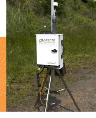
We've designed a NJDEP PAM Monitoring package using the latest in hardware and software technology to make monitoring easy. Weatherproof monitors arrive fully assembled, with tripod, 15-hour lightweight battery pack and connection to Aeroqual cloud for automated data collection, presentation, alerts and PDF reporting.
